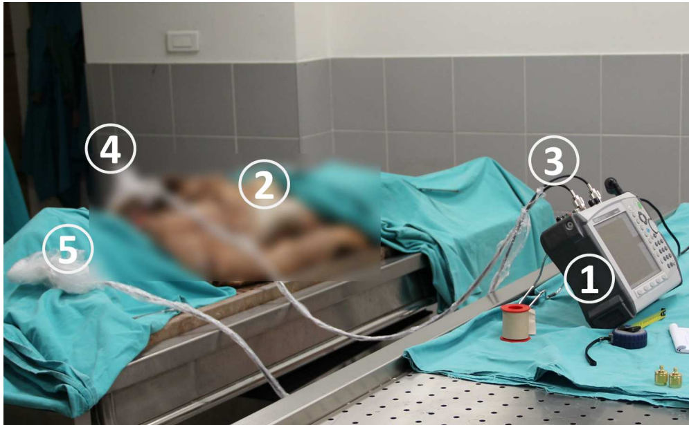
Figure 3.3: Experiment setup for the in vivo channel: 1) Vector network analyzer (VNA), 2) human male cadaver, 3) coaxial cables, 4) a novel tapered slot CPW-fed antenna ( in vivo ), 5) insulated dipole antenna ( ex vivo ).
